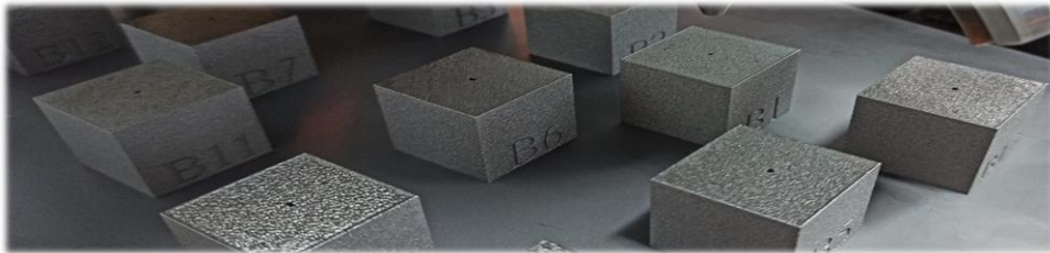
Figure 4-58 Exposure time, volumetric energy density, point distance, hatch distance effect investigation DOE-II samples
