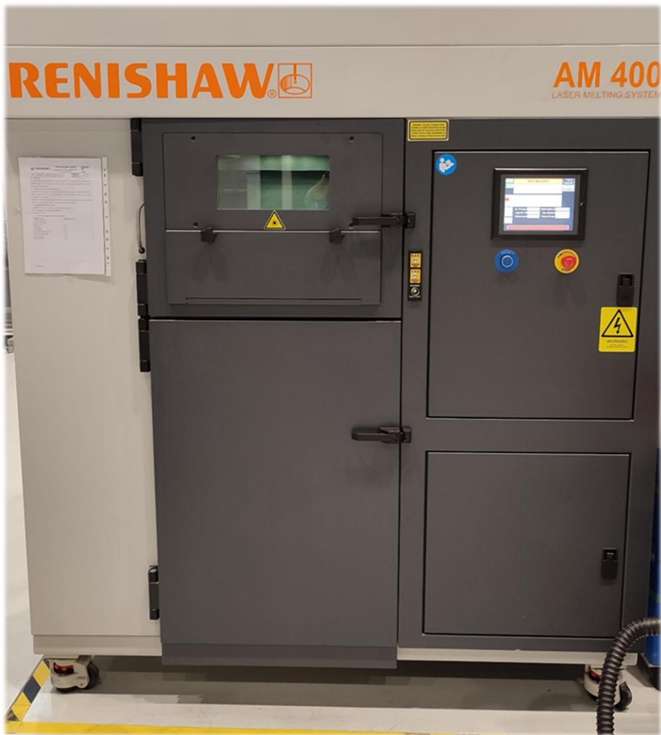
Figure 3-4 Renishaw AM400 laser powder bed fusion additive manufacturing equipment
