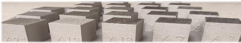
Figure 4-53 Power, point distance, hatch distance effect investigation DOE-I samples
